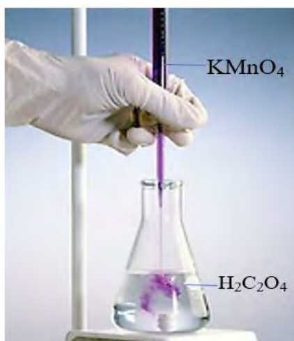
Fig: Redox titration between potassium permanganate and oxalic acid solution
