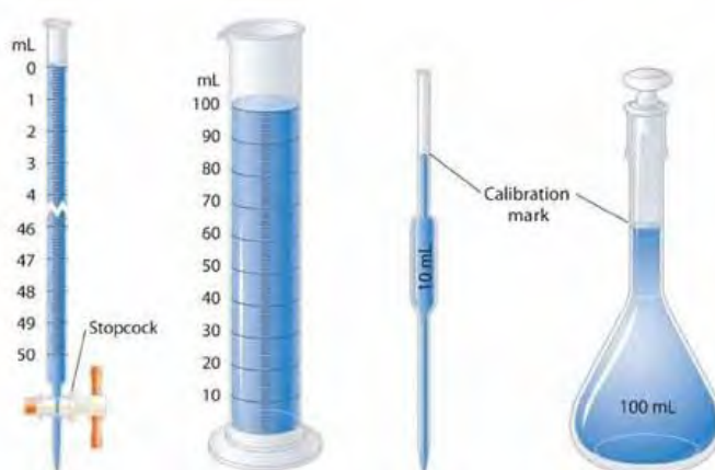
Figure: Glasswares for measuring volume of liquid (burette, measuring cylinder, pipette and volumetric flask)
